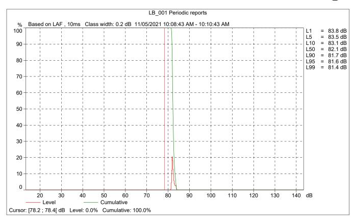
Site Number: NM-2 Recorded By: Danielle Regimbal, Tina Yuan **Job Number:** 178554 **Date:** 11/5/2021 **Time:** 10:13 AM Location: 5 feet from rear diver side of the truck Source of Peak Noise: Trucks idling and trenching events Noise Data Leq (dB) Lmax(dB) Lmin (dB) Peak (dB) 90.3 95.0 78.0 107.3
