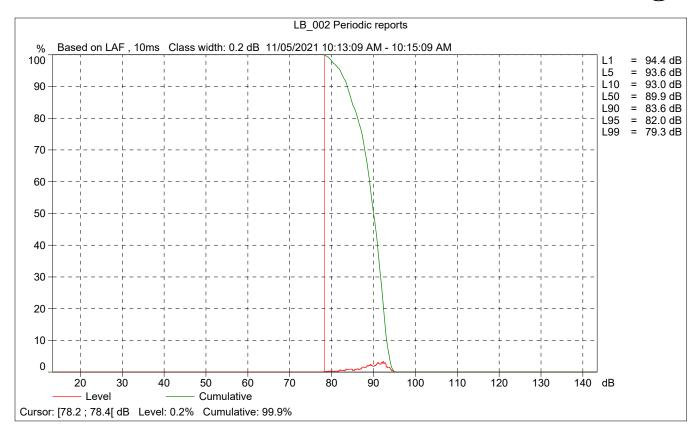
Site Number: NM-3 Recorded By: Danielle Regimbal, Tina Yuan **Job Number:** 178554 Date: 11/5/2021 **Time:** 10:17 AM Location: 5 feet from the rear passenger side Source of Peak Noise: Trucks idling and trenching events Noise Data Leq (dB) Lmax(dB) Lmin (dB) Peak (dB) 88.0 101.5 80.3 110.0
