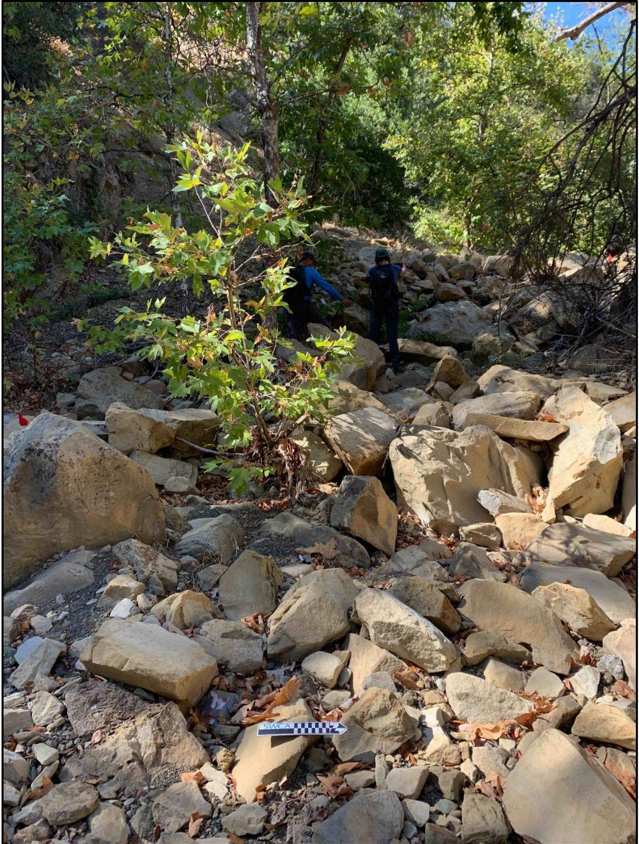
**Figure 17. Sidecast material of Coldwater Formation (Tsw) situated along the Mission Canyon slope south of Road Area 4.**
