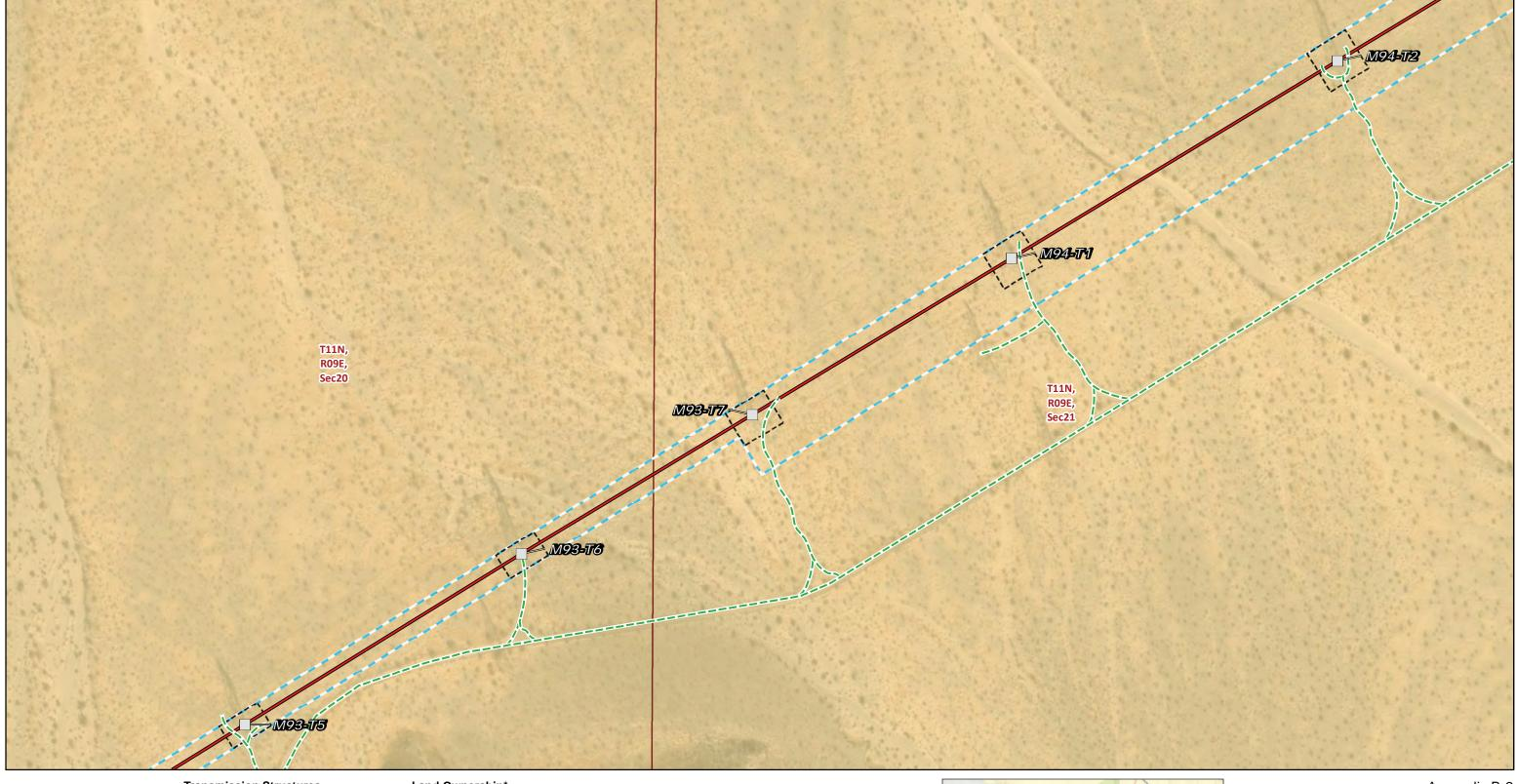
Transmission Structures Existing Transmission Towers Existing Access Roads Access Road Transmission New Optical Ground Wire Overhead Construction Areas Structure Work Area Right of Way
