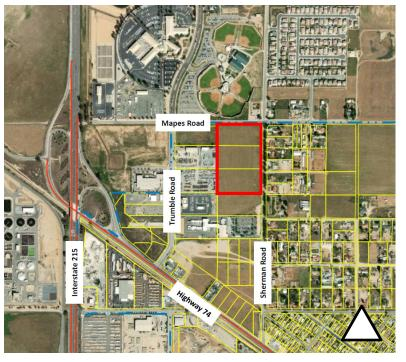
**Plot Plan No. PLN22-015** proposes to construct an approximately 277,578 square foot (sq. ft.) concrete tilt-up building, which includes 10,000 sq. ft. of office space on a vacant 13.34 gross acre project site. The proposed building would have a maximum overall height of approximately 51 feet and include 36 dock-high doors. The project also includes 308 proposed parking spaces, on-site landscape and full on-site and off-site improvements.
