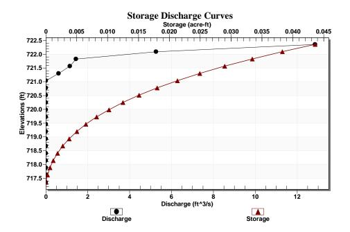
Figure 4: Storage discharge curves calculated for Attenuation Basin 2.
