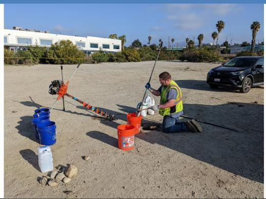
**PHOTO 5:** Hand augering being performed at Boring B-09.
