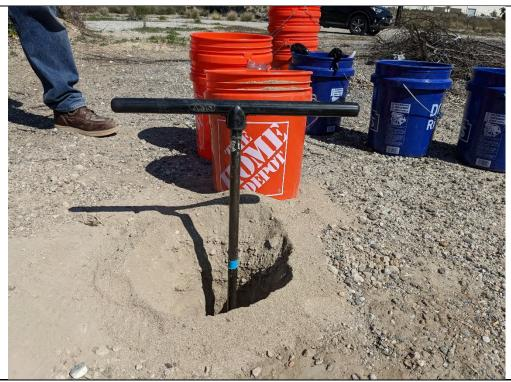
PHOTO 4: View of hand auger ready to collect sample B-03-4.
