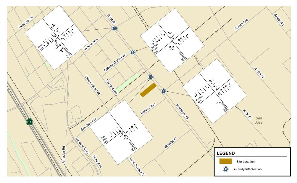
Figure 6 Existing Intersection Lane Configurations
