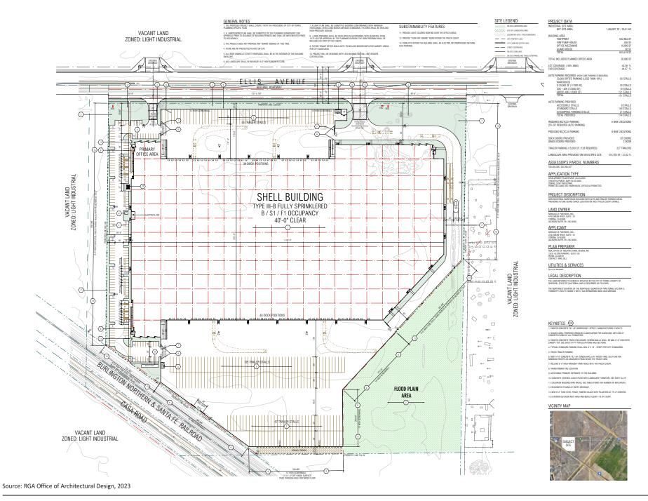
Figure 2-5: Proposed Site Plan
