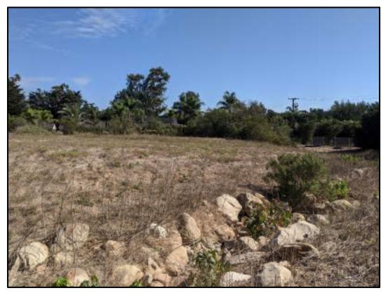
Photo 4. Evidence of imported fill soils within Proposed Lot 1, looking east.  $$\mathbf{2}$$
