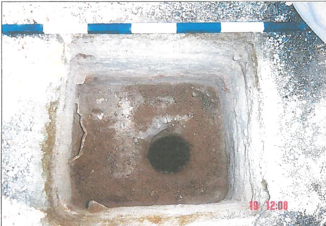
Photo 2: East wall of Test Unit 55 at the far end of the NPS-owned portion of the Oasis of Mara. Side wall Shows the ore mill tailings deposit at this location. This area is the location of several ore mills that operated At the Oasis of Mara in the late 19<sup>th</sup> century. Scale in 10-cm increments.
