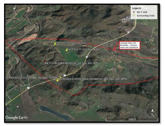
Figure 4. Surrounding Wells in the Same Geologic Unit
