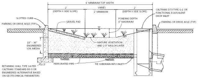
While the 18-inch minimum engineered soil media depth can be used in some cases, it is recommended to use 24 inches or a preferred 36 inches to provide an adequate root zone for the chosen plant palate. Such a design also provides for improved removal effectiveness for nutrients. The recommended ponding depth inside of a Bioretention Facility is 6 inches; measured from the flat bottom surface to the top of the water surface as shown in Figure 1.
