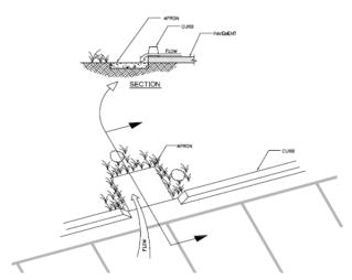
Figure 3: Apron located in a Bioretention Facility
