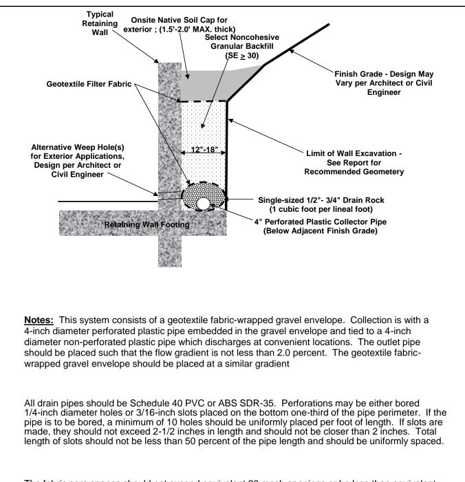
The fabric pore spaces should not exceed equivalent 30 mesh openings or be less than equivalent 100 mesh openings. The fabric should be placed such that a minimum lap of 8-inches exists at all splices.
