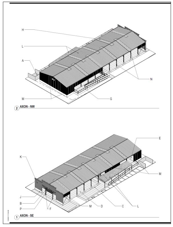
Figure 25. 3D site plans showing the west and east elevations, with the new concrete loading docks, which will also comply with ADA.
