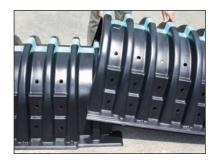
Directional arrows located on the top of the chamber point towards the Small Rib End. The open end of the next chamber overlaps the small rib end of the preceding chamber.
