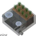
minimizes the system length, providing a highly compact footprint. It has been proven useful in situations such as streets with directly adjacent sidewalks, as half of the system can be placed under that sidewalk. This orientation also offers internal bypass options as discussed below.
