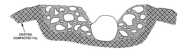
EXCAVATE HOLE INTO EXISTING FILL PRISM, PLACE BOULDER (< 8 feet in maximum dimension) INTO EXISTING COMPACTED FILL. SURROUND WITH SAND, GRAVEL, COBBLES AND WATER HEAVILY. TRACK WITH D8 OR LARGER EQUIPMENT UNTIL RESULTING FILL FULLY SUPPORTS EQUIPMENT. OBSERVE AND/OR TEST IN ACCORDANCE WITH ASTM D1556, D2922 OR D3017. ROCKS LARGER THAN 8 FEET SHALL BE FURTHER REDUCED IN SIZE BY SECONDARY BREAKING.
