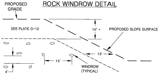
NOTE: OVERSIZED MATERIAL SHOULD BE REMOVED FROM THE 15'
