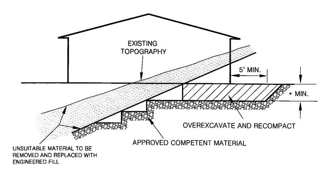
\*NOTE ALL BUILDING PADS SHALL BE OVER EXCAVATED TO A MINIMUM OF 1/3 OF THE MAXIMUM DEPTH OF FILL BELOW THE BUILDING PAD TO A MAXIMUM OF 17 FEET (SEE PLATE G-16)
