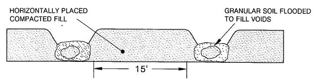
NOTE: COMPACTED FILL SHALL BE BROUGHT UP TO A HIGHER ELEVATION ALONG EACH WINDROW SO GRANULAR SOIL CAN BE FLOODED IN A "TRENCH CONDITION".
