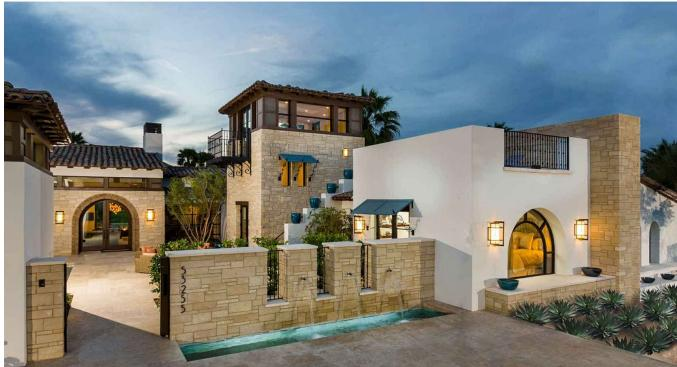
1. Smooth plaster, stone veneer, clay tile roofing, steel or iron rails, ceramic pots, canvas awnings, stone or tile paving, landscaping.
