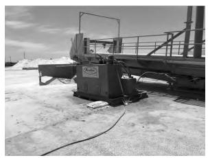
Photo #23 View of the above ground hydraulic power source for the tipper containing diesel fuel and hydraulic oil.
