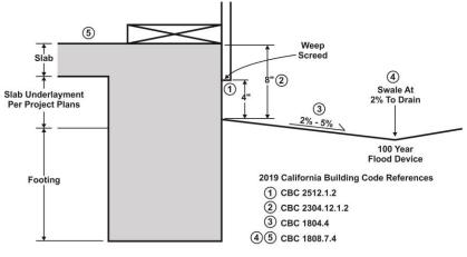
Typical 2019 California Building Code Drainage Requirements
