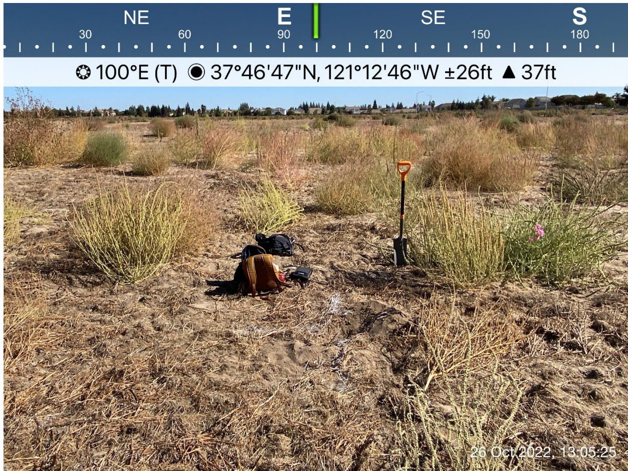
Photo 5: Sampling point A located outside of the NWI riverine (south) at 37.780030, -121.212870. The ground was littered with dead/uprooted vegetation due to what appeared to be tilled soil. No wetland indicators were met, and this area is not considered a wetland.
