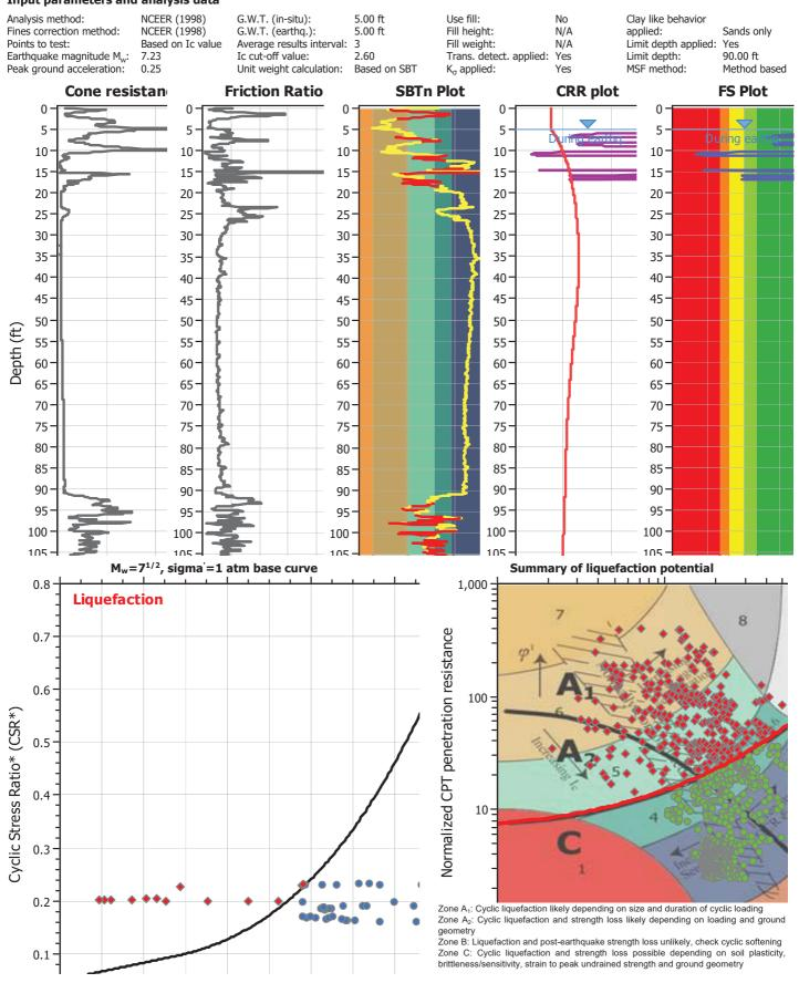
CLiq v.3.3.3.4 - CPT Liquefaction Assessment Software - Report created on: 1/12/2022, 4:44:05 PM Project file: G:\Active Projects\\_18000 to 19999\19542\19542000001\Analysis\Liquefaction\Alameda Ferry Terminal - CLE.clq
