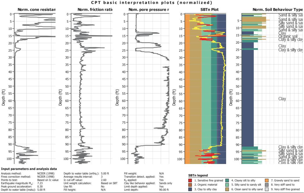
CLiq v.3.3.3.4 - CPT Liquefaction Assessment Software - Report created on: 1/12/2022, 4:41:13 PM Project file: G:\Active Projects\\_18000 to 19999\19542\1954200001\Analysis\Liquefaction\Alameda Ferry Terminal - CLE.clq 2
