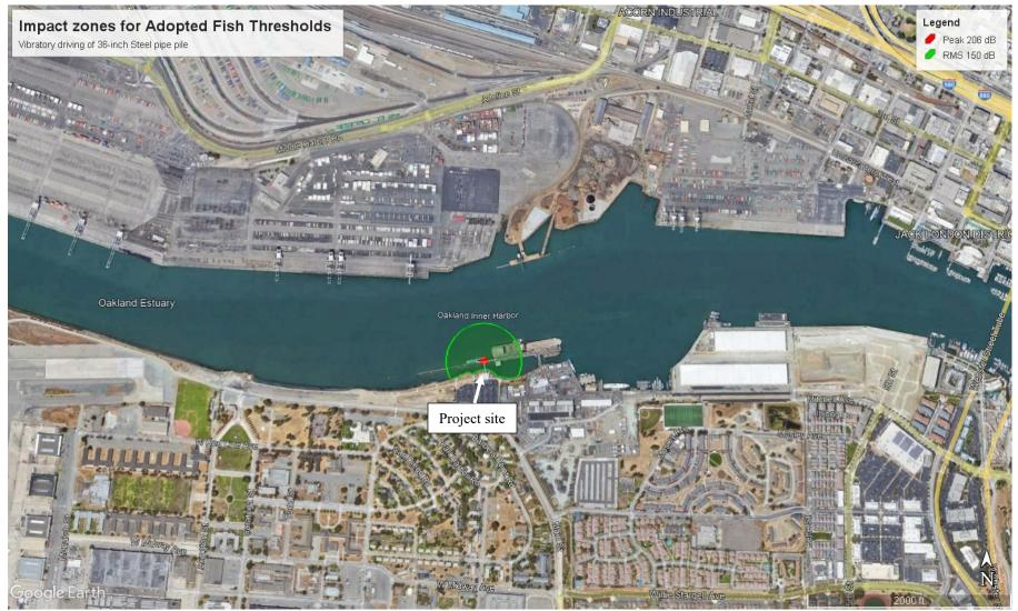
Figure A5 – Fish Injury Zones – 206 dB Peak, 150 dB RMS and 187 SEL<sub>cum</sub>; for 36-inch Steel pile driven using a vibratory hammer
