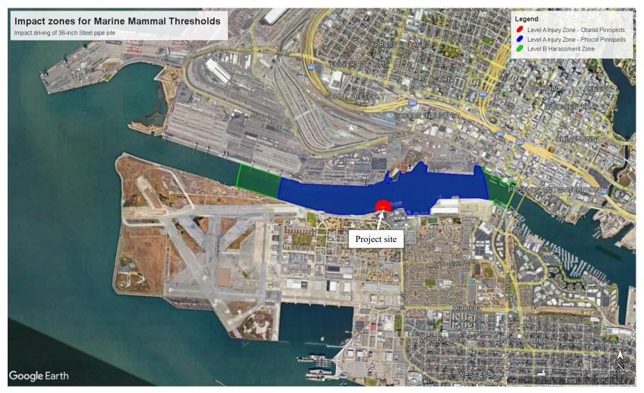
Figure A8 – Marine Mammal Level A and B Zones – Phocid and Otariid Pinnipeds; for 36-inch Steel pile impact driven
