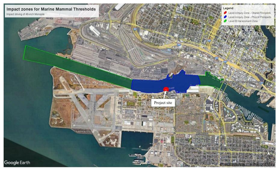
Figure A9 – Marine Mammal Level A and B Zones – Phocid and Otariid Pinnipeds; for 48-inch monopile impact driven
