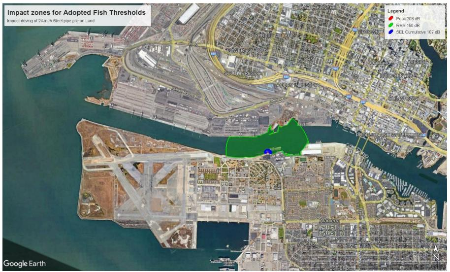
Figure A1 – Fish Injury Zones – 206 dB Peak, 150 dB RMS and 187 SEL<sub>cum</sub>; for 24-inch Steel pile on Land impact driven
