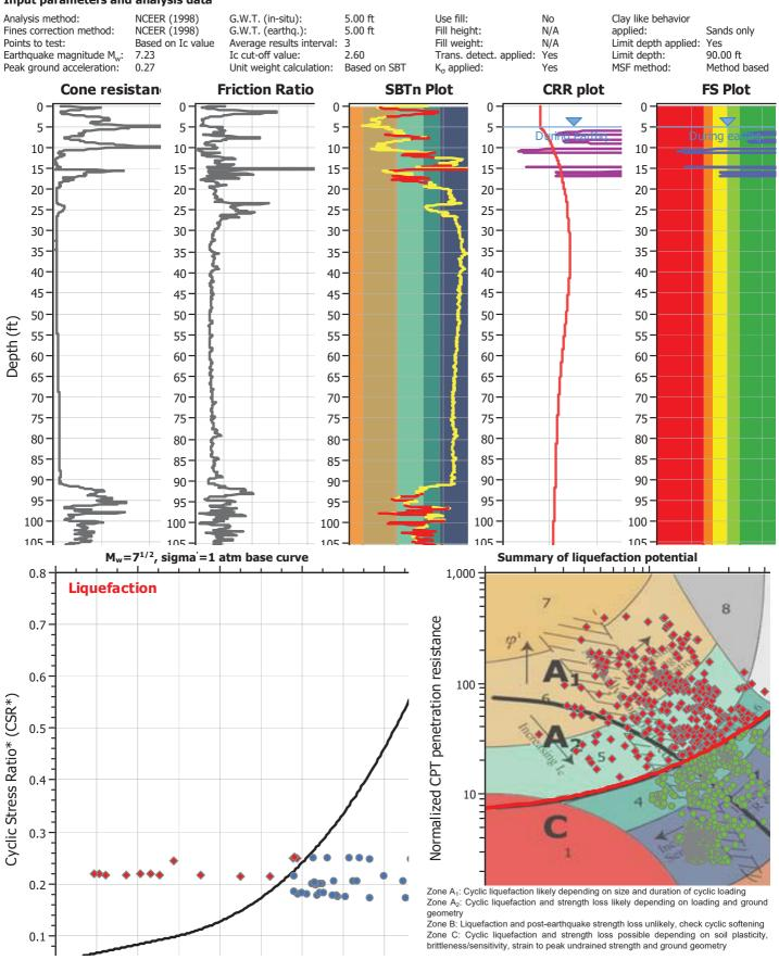
CLiq v.3.3.3.4 - CPT Liquefaction Assessment Software - Report created on: 1/12/2022, 4:46:58 PM Project file: G:\Active Projects\\_18000 to 19999\19542\1954200001\Analysis\Liquefaction\Alameda Ferry Terminal - CLE.clq
