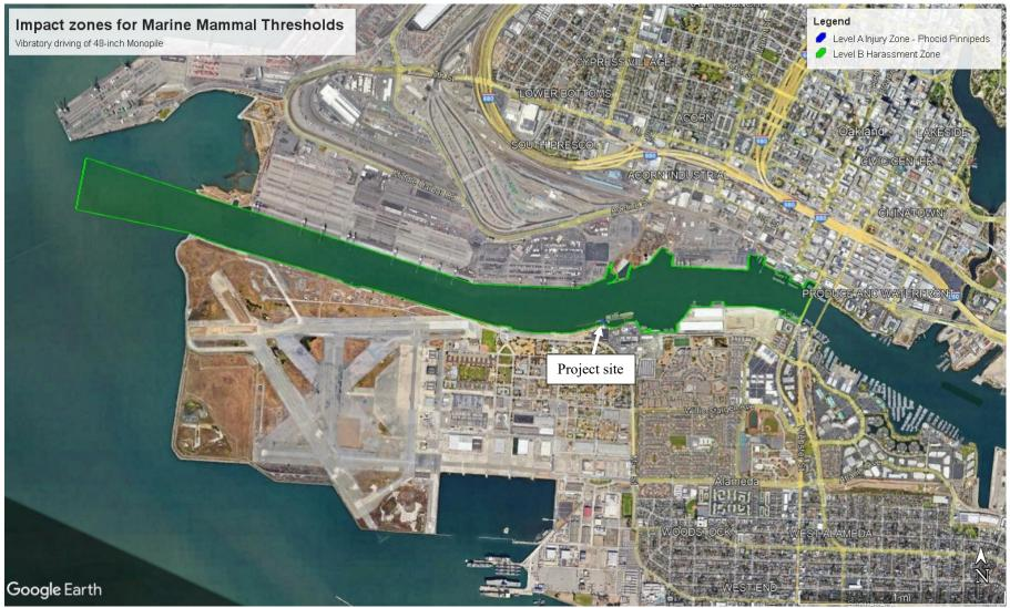
Figure A12 – Marine Mammal Level A and B Zones – Phocid and Otariid Pinnipeds; for 48-inch monopile driven using a vibratory hammer
