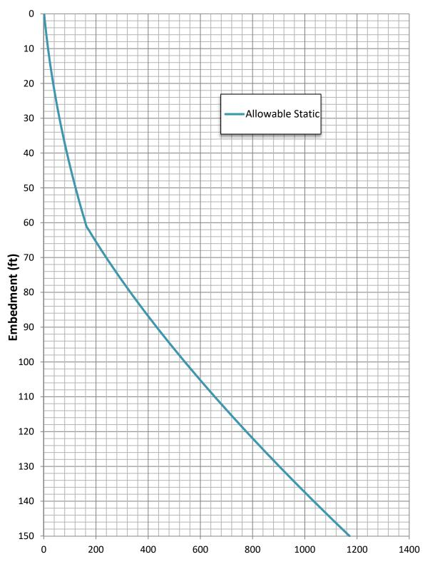
Allowable Axial Capacity (kips)
