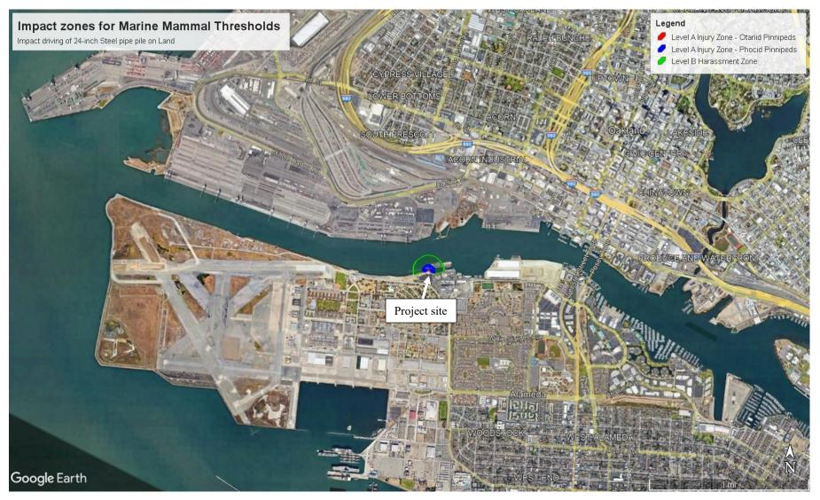
Figure A7 – Marine Mammal Level A and B Zones – Phocid and Otariid Pinnipeds; for 24-inch Steel pile on Land impact driven
