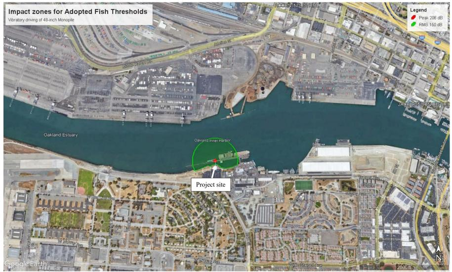
Figure A6– Fish Injury Zones – 206 dB Peak, 150 dB RMS and 187 SEL<sub>cum</sub>; for 48-inch monopile driven using a vibratory hammer
