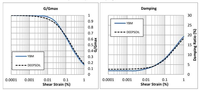
EXHIBIT 10: Modulus Reduction (G/Gmax) and Damping Curves for YBM and the DEEPSOIL fit
