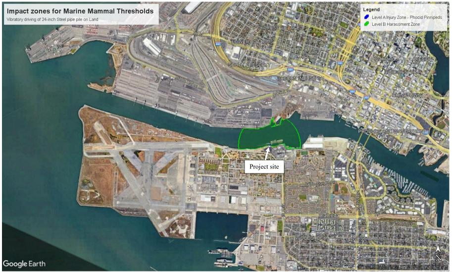
Figure A10 – Marine Mammal Level A and B Zones – Phocid and Otariid Pinnipeds; for 24-inch Steel pile on Land driven using a vibratory hammer
