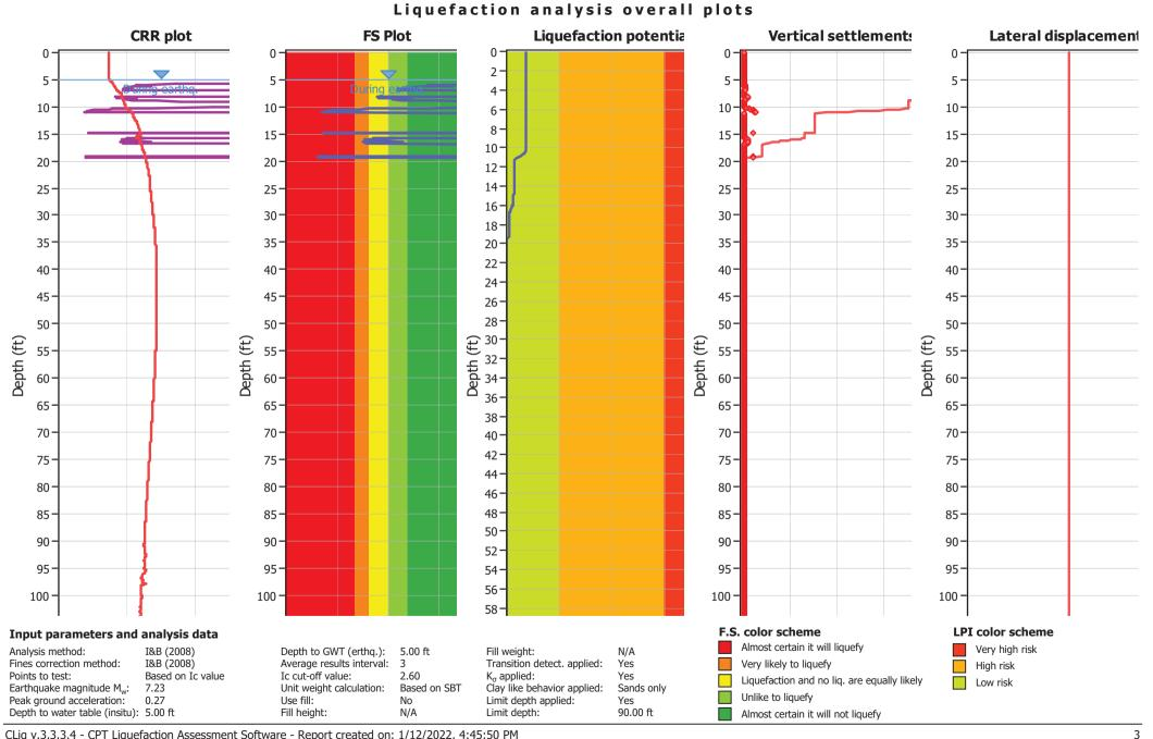
CLiq v.3.3.3.4 - CPT Liquefaction Assessment Software - Report created on: 1/12/2022, 4:45:50 PM Project file: G:\Active Projects\\_18000 to 19999\19542\19542000001\Analysis\Liquefaction\Alameda Ferry Terminal - CLE.clq
