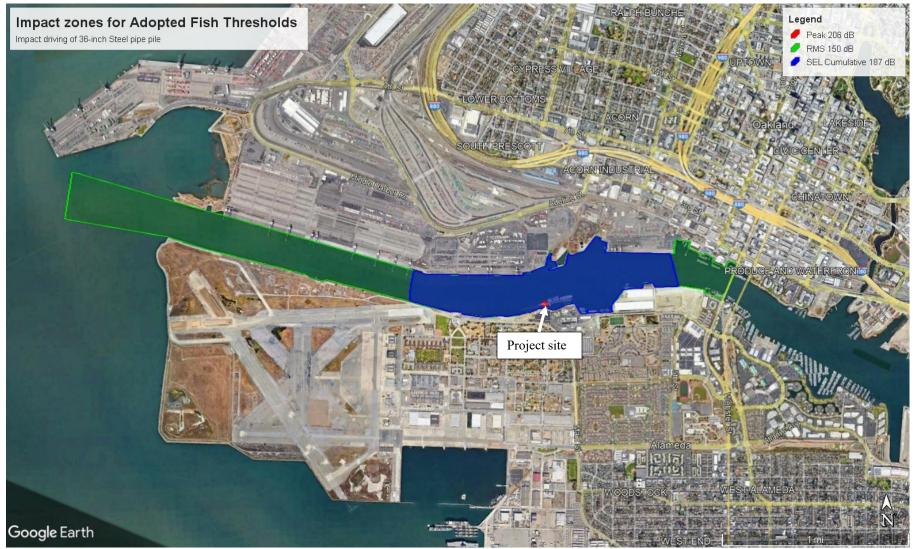
Figure A2 – Fish Injury Zones – 206 dB Peak, 150 dB RMS and 187 SEL<sub>cum</sub>; for 36-inch Steel pile impact driven
