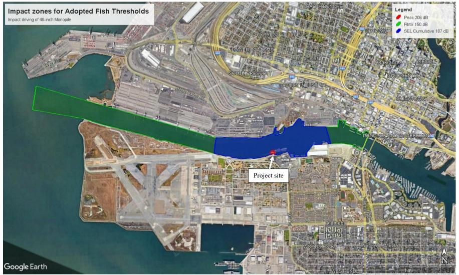
Figure A3 – Fish Injury Zones – 206 dB Peak, 150 dB RMS and 187 SEL<sub>cum</sub>; for 48-inch monopile impact driven
