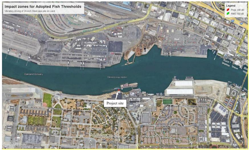
Figure A4 – Fish Injury Zones – 206 dB Peak, 150 dB RMS and 187 SEL<sub>cum</sub>; for 24-inch Steel pile on Land driven using a vibratory hammer
