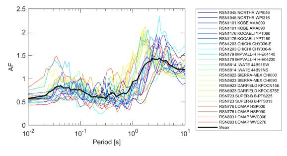
Offshore Non-Liquefiable Profile DE Scenario
