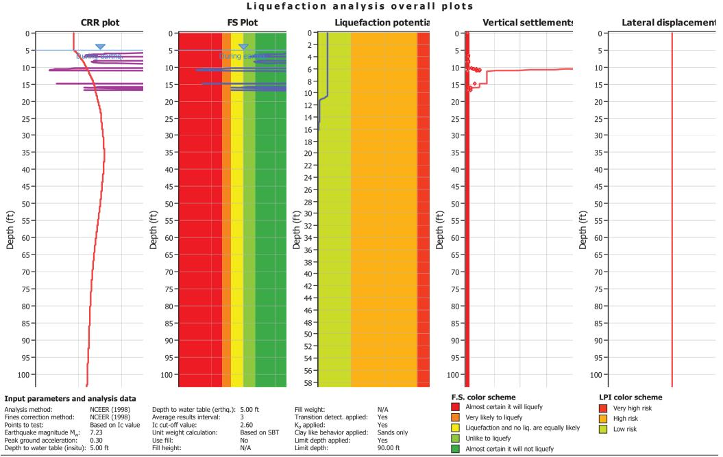
CLiq v.3.3.3.4 - CPT Liquefaction Assessment Software - Report created on: 1/12/2022, 4:41:13 PM Project file: G:\Active Projects\\_18000 to 19999\19542\1954200001\Analysis\Liquefaction\Alameda Ferry Terminal - CLE.clq
