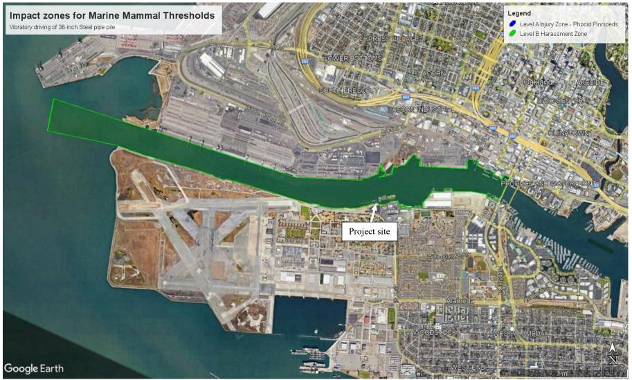
Figure A11 – Marine Mammal Level A and B Zones – Phocid and Otariid Pinnipeds; for 36-inch Steel pile driven using a vibratory hammer
