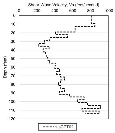
Based on the measured  $V_{S30}$ , we classified the site as borderline Site Class E. However, due to presence of the loose sandy material below the estimated groundwater table (about 5 feet below ground surface), the site is characterized as potentially liquefiable and is classified as a Site Class F.
