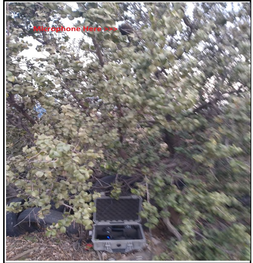
LTNM1 looking N, showing location of equipment on ground & location of microphone in tree. Microphone about 7 feet above the ground.
