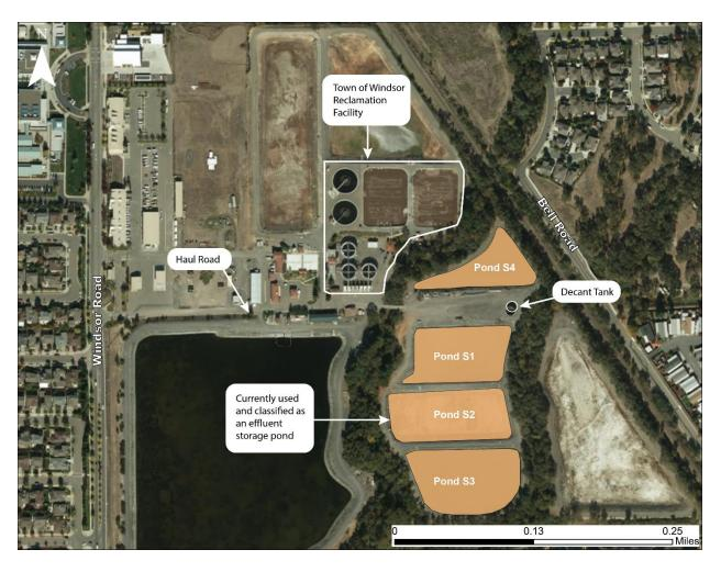
Figure 2-3. Existing Sludge Storage Ponds
