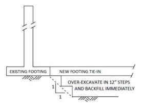
Maintaining a sufficient clear distance between new and existing foundations will reduce the potential for
