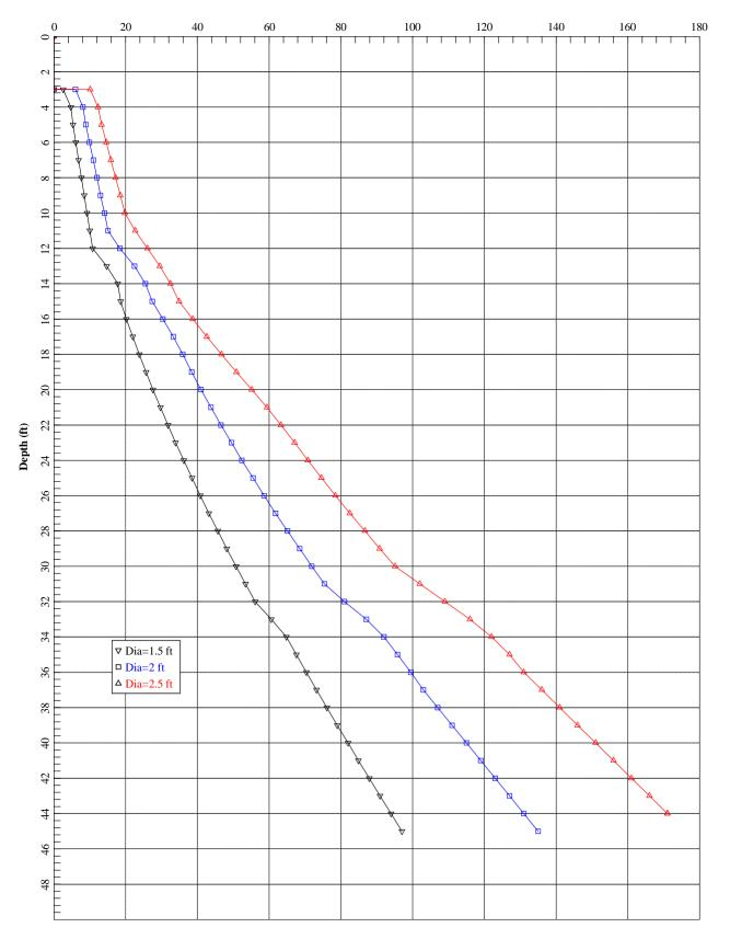
Allowable Side Resistance Side Resistance/F.S. (tons)
