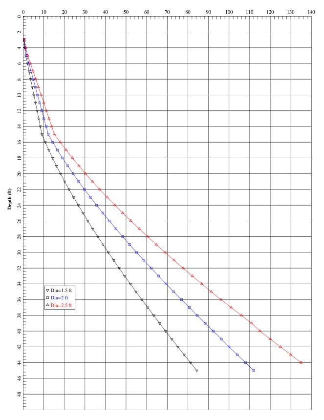
Allowable tension capacity may be taken as 60 percent of the allowable Side Resistance capacity shown in the graph, plus the weight of the pile.
