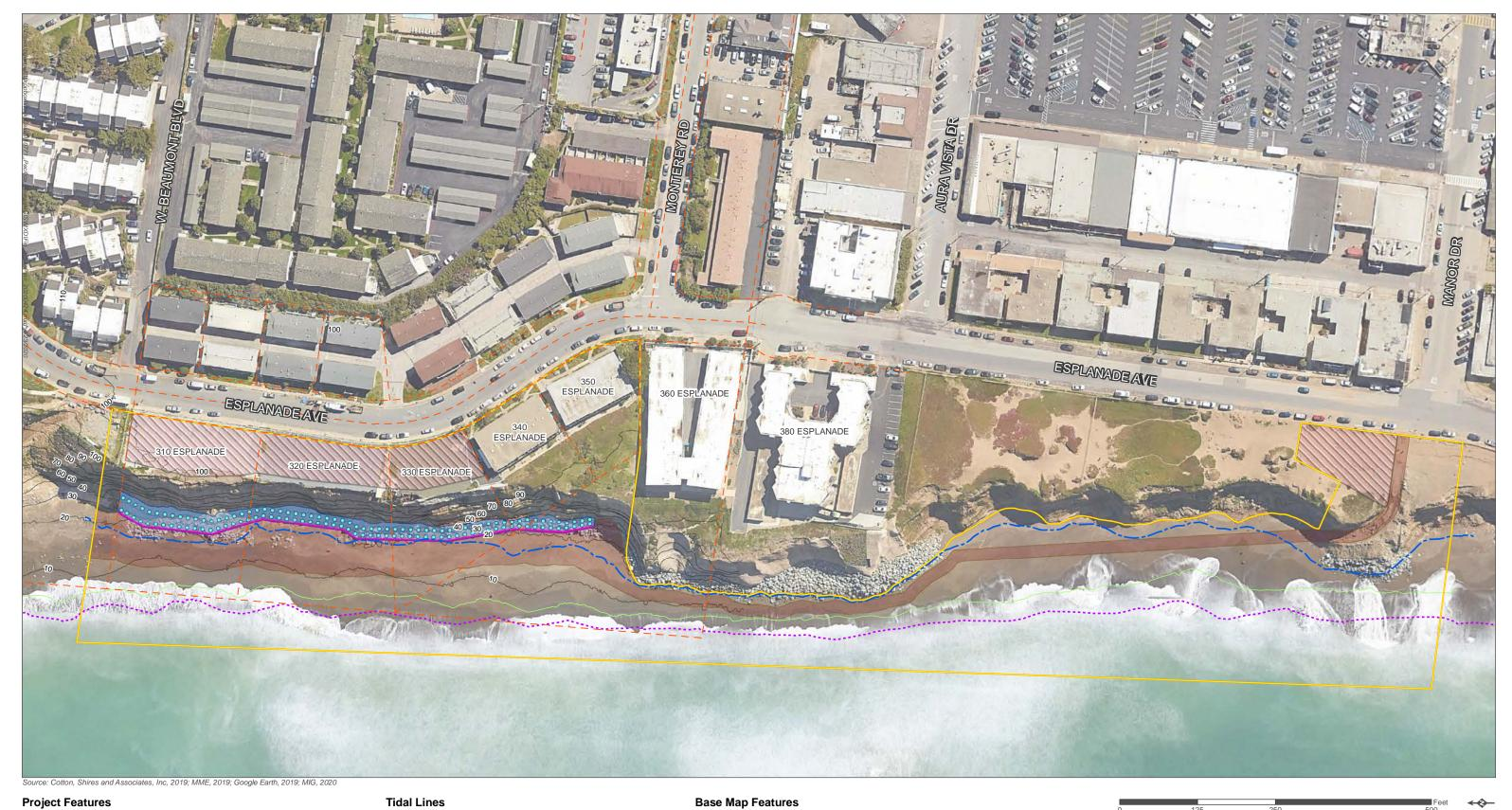
Study Area --- High Tide Line (HTL)1 Proposed Seawall Highest Astronomical Tide (HAT)<sup>2</sup>, 7.32 ft NAVD88 Staging Area Proposed Pile Cap Temporary Construction Access ····· Mean High Water (MHW)<sup>3</sup>, 5.29 ft NAVD88 Proposed Tieback MIG, 2019, 2020
