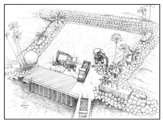
Figure 8. Illustration of Island Pavement Removal
