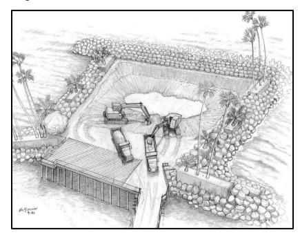
Figure 10. Illustration of Contaminated Soil Removal
