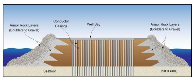
Figure 6. Rincon Island Cross Section (Illustration)
