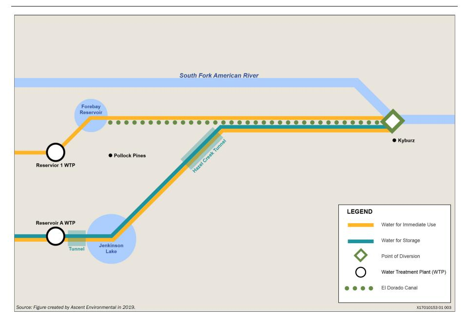
Figure 5 Water Diversion from El Dorado Diversion Dam
