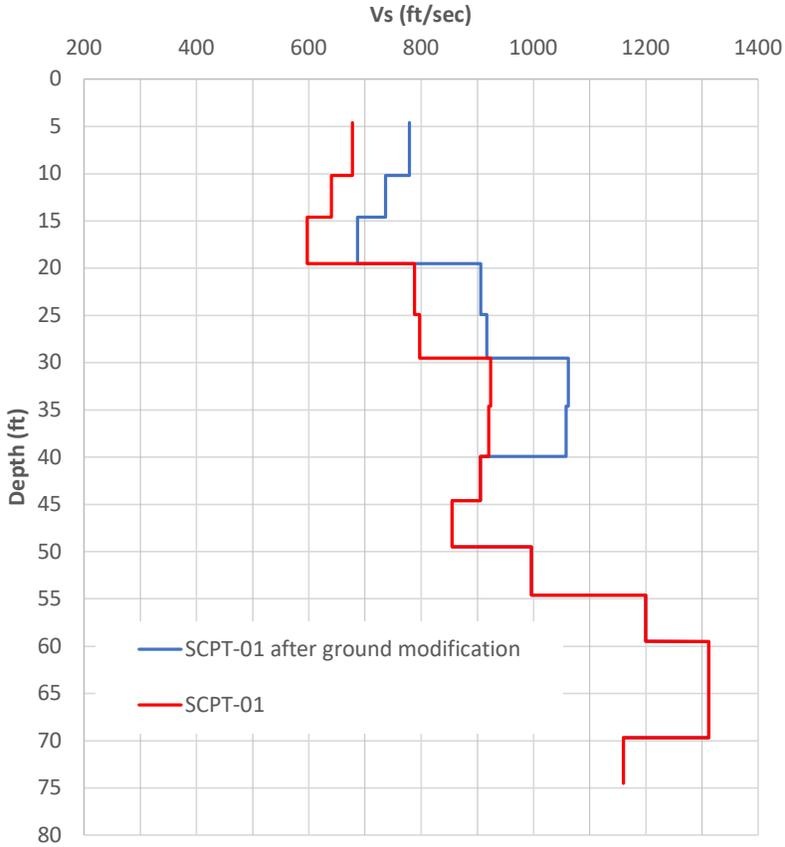
Figure 1: Shear Wave Velocity Profiles
