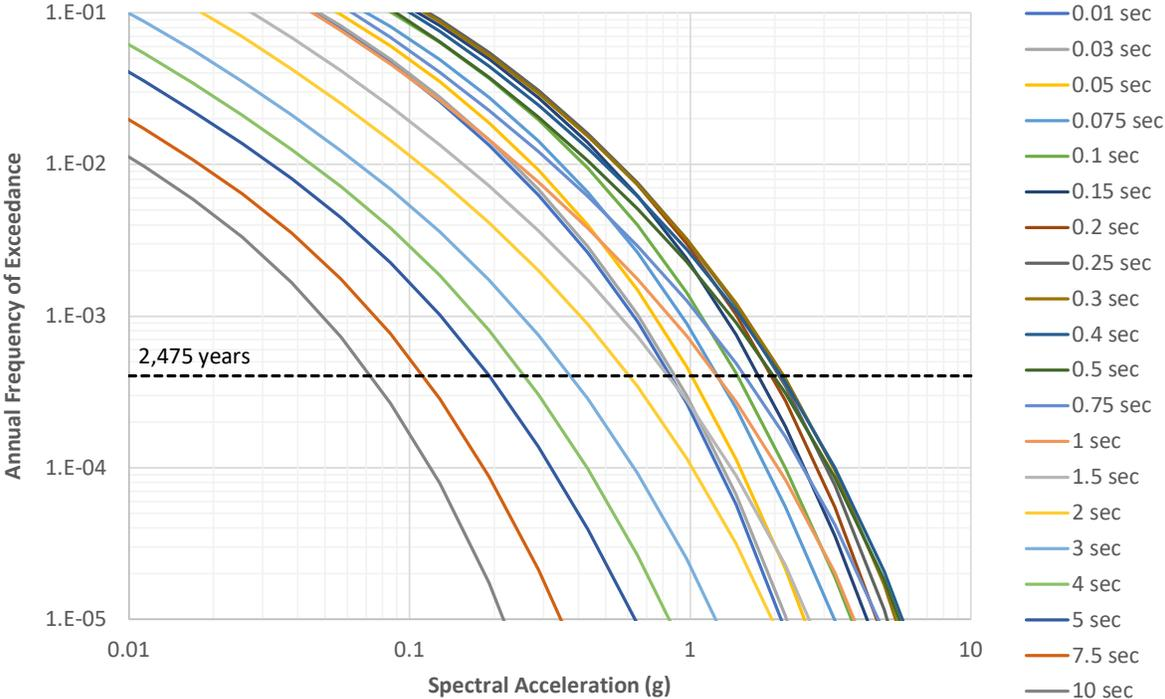
Figure 2: Mean Annual Seismic Hazard Curves for Vs30 of 310 m/s
