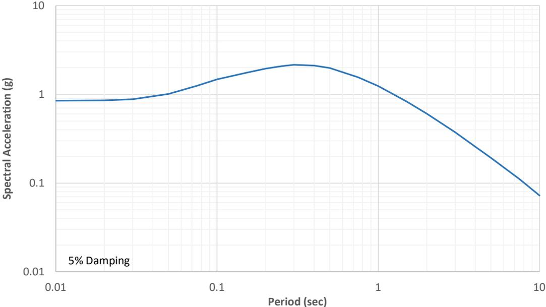
**Figure 3: Mean Horizontal Uniform Hazard Response Spectrum for a Return Period of 2,475 Years and Vs30 of 310 m/s**
