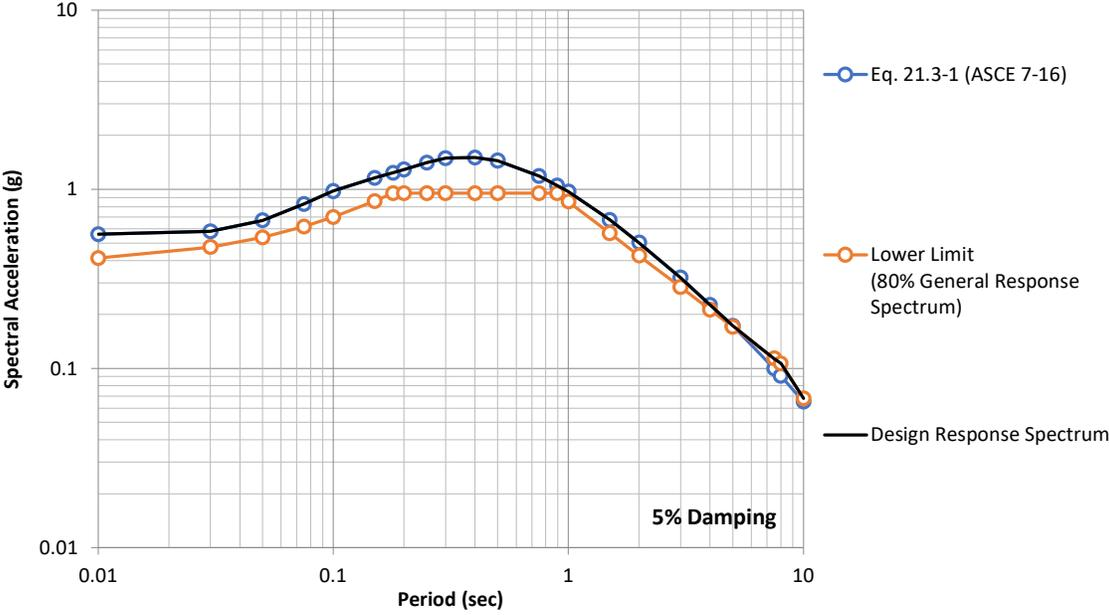
Figure 5: Calculation of the Site-Specific Horizontal MCE\_R and Design Response Spectra per ASCE 7-16 for Vs30 of 310 m/s
