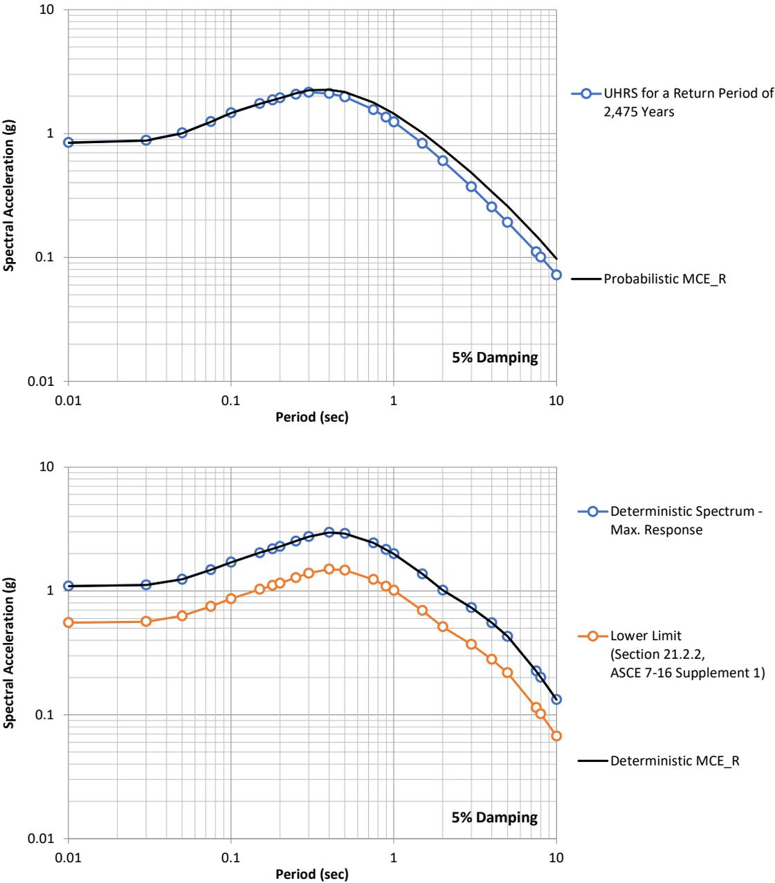
**Figure 4: Calculation of the Probabilistic and Deterministic Horizontal MCE\_R Response Spectra per ASCE 7-16 for Vs30 of 310 m/s**
