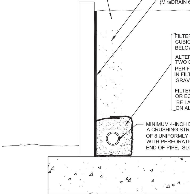
FILTER MATERIAL - MINIMUM OF TWO CUBIC FEET PER FOOT OF PIPE. SEE BELOW FOR FILTER MATERIAL SPECIFICATION.
