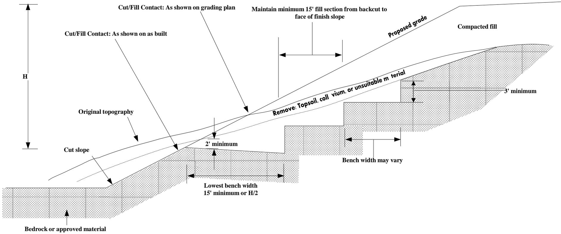
Note: The cut section shall be excavated and evaluated by the soils engineer/engineering geologist prior to constructing the fill portion.
