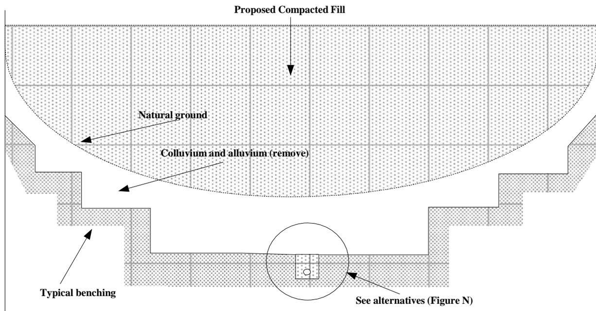
Note: Alternatives, locations, and extent of subdrains should be determined by the soils engineer and/or engineering geologist during actual grading.
