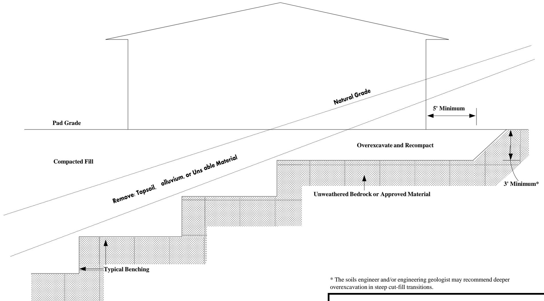
\* The soils engineer and/or engineering geologist may recommend deeper overexcavation in steep cut-fill transitions.
