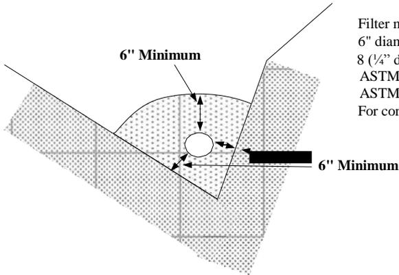
Filter material: Minimum volume of 9 feet<sup>3</sup>/linear foot.
