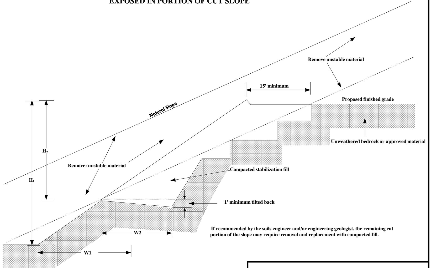
If recommended by the soils engineer and/or engineering geologist, the remaining cut portion of the slope may require removal and replacement with compacted fill.
