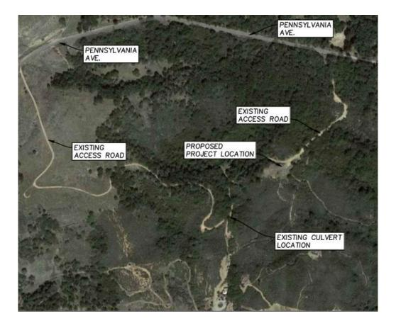
The existing culvert must have the capacity to convey runoff from a 25-year storm event per county of Santa Barbara Flood Control Standard Conditions.
