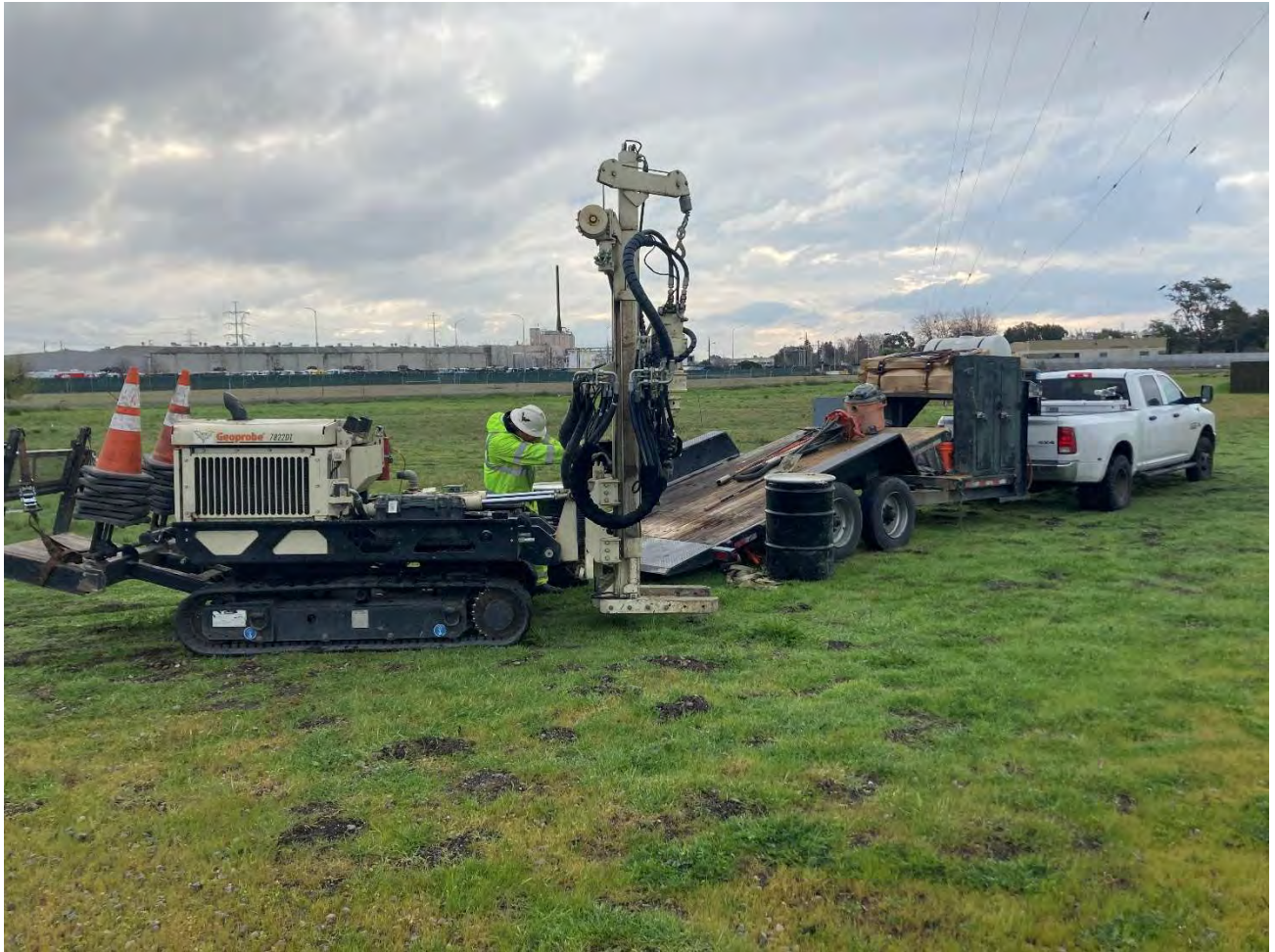
Photo 1 – Setting-up GeoProbe at Borehole DSB-1
