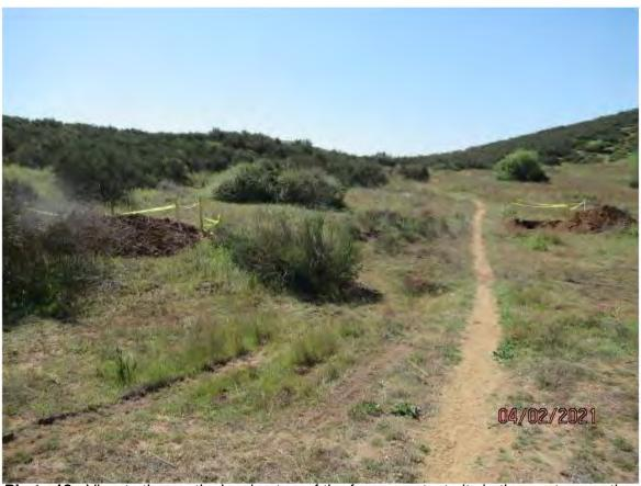
**Photo 12** - View to the south showing two of the four open test pits in the western portion of the subject site believed to have been used for recent double ring infiltration testing.
