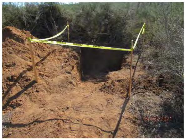
**Photo 13** - Closeup view of one of the four test pits within the western portion of the subject site believed to have been used for recent double ring infiltration testing.
