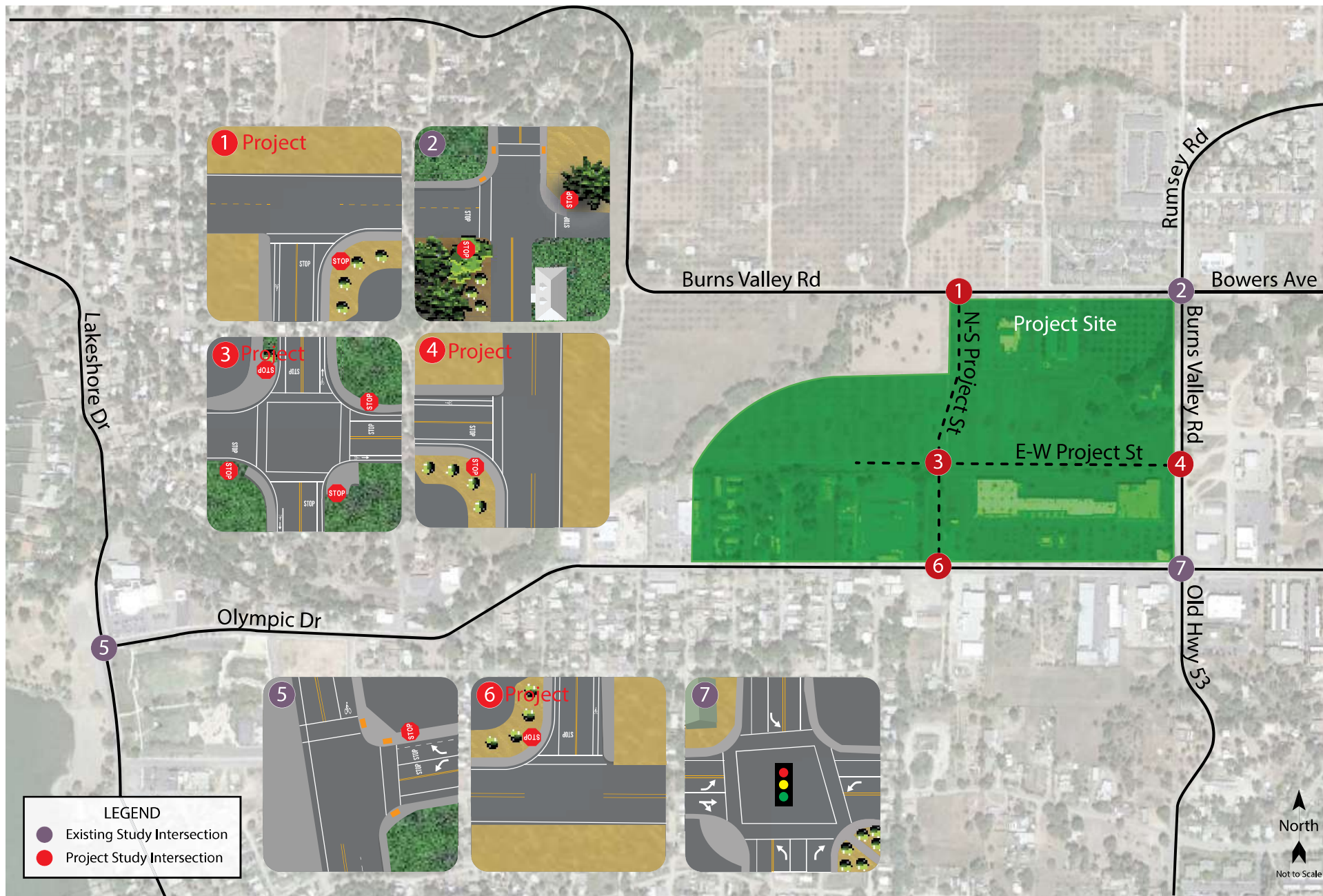
Transportation Impact Study for the Burns Valley Development Figure 1 – Study Area, Existing and Proposed Lane Configurations
