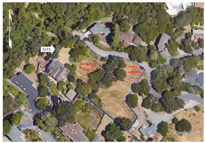
Photo 1: Aerial view from April 2018 of the subject property to the left and 634 Palomar Drive to the right. The landslide repair is visible on the subject property and an active landslide is apparent on 634 Palomar Drive.
