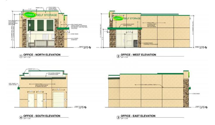
Figure 6 – Building B Elevations
