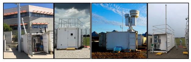
• (1) ARM Support Container for storing tools, gear, consumables, spare parts/instruments, etc. to service the instruments and equipment on the research containers. This is a typical 8.5' high container with no roof attachments.
