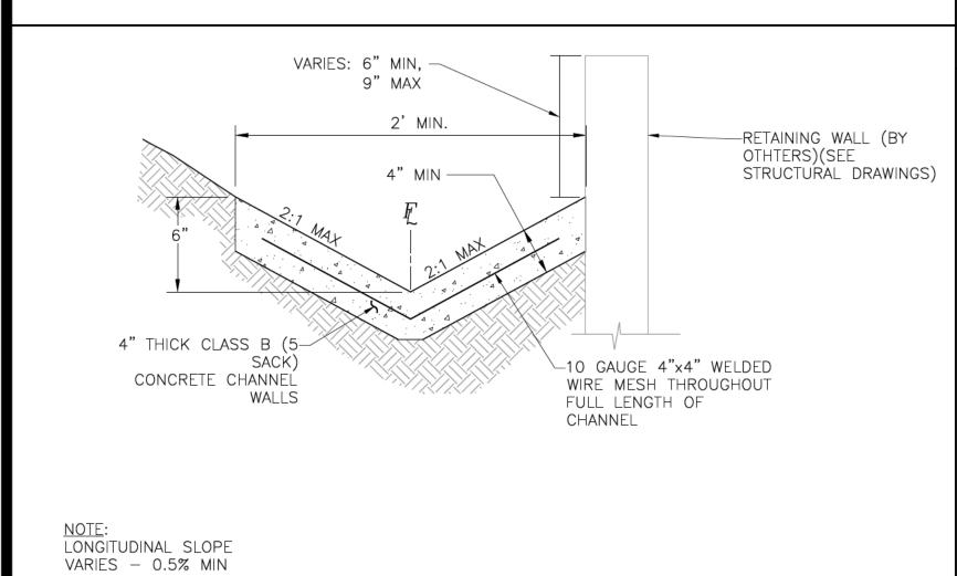
B FIELD DRAIN W/ TRIANGULAR SO DETAIL
