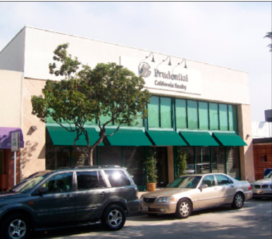
2. Single-Bay Frame. This architectural expression focuses on the pattern of a structural frame defining a single opening to the street. This opening is part of a commercial storefront frontage. Its glazing and bulkhead design can be slightly inset from the street, slightly inset to define an entrance pocket, or deeply inset to define an outdoor sitting area.
