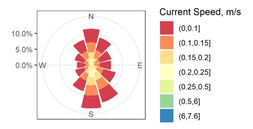
**Figure 3.** Current speed and direction measurements at the SBOO for total period of record (August 2018 to November 2020). Radius represents fraction of measurements within that speed and direction category.
