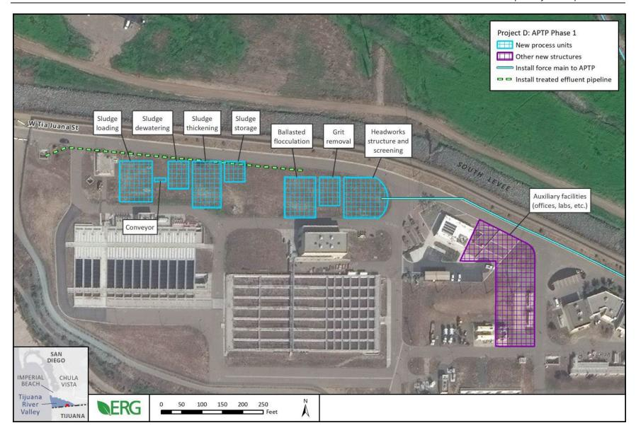
Figure 1-9. Project D (APTP Phase 1) – Conceptual Site Plan of Proposed Facilities
