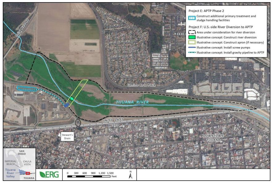
Figure 2-1. Projects E (APTP Phase 2) and F (U.S.-side River Diversion to APTP) - Conceptual Locations of Project Components
