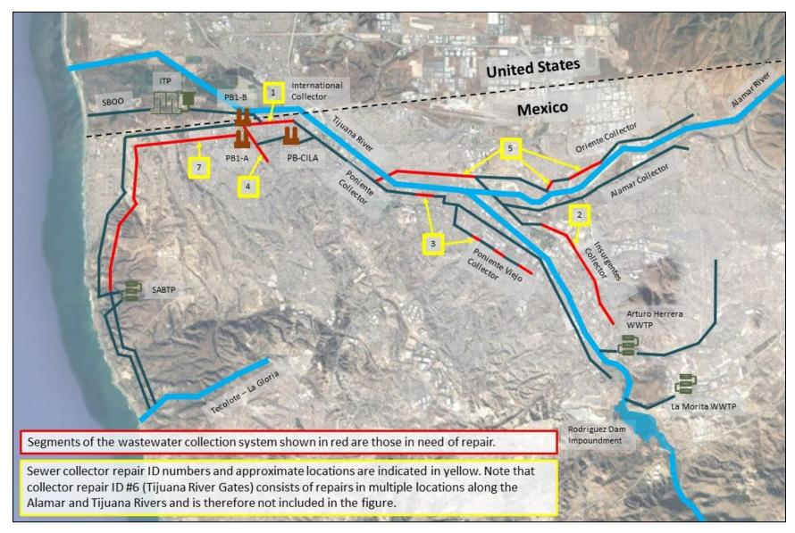
Figure 1-6. Project C – Schematic of Tijuana Sewer Collectors for Rehabilitation or Replacement
