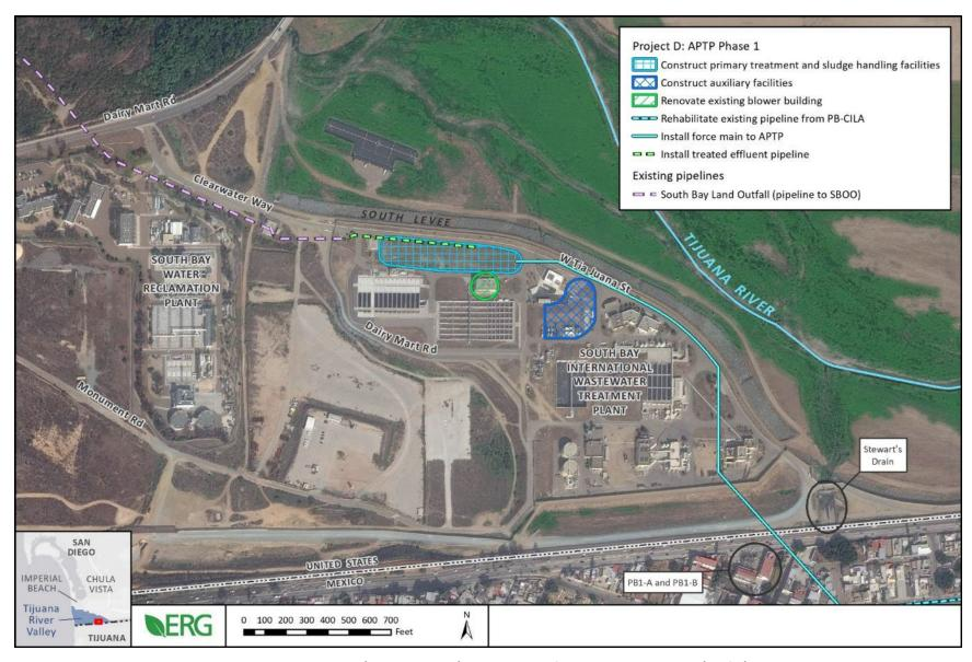
Figure 1-7. Project D (APTP Phase 1) – Locations of Project Components (1 of 2)
