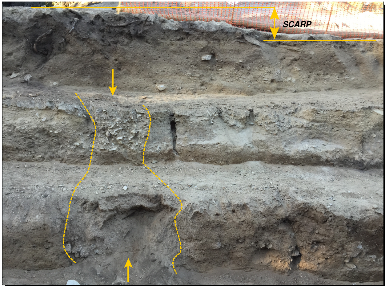
Fault trench FT-1, view north at “main trace” of Glen Ivy South fault zone. Chimney-like fissure fills transect the 25-foot width of the excavation, trending almost perpendicular to apical fan stream flow direction. Noted topographic scarp continues beyond the image through a native oak grove before becoming obscured by a man-made irrigation water basin.
