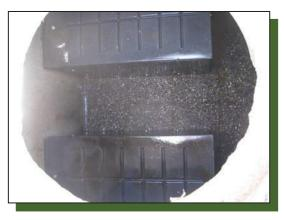
Fully cleaned separation chamber.
