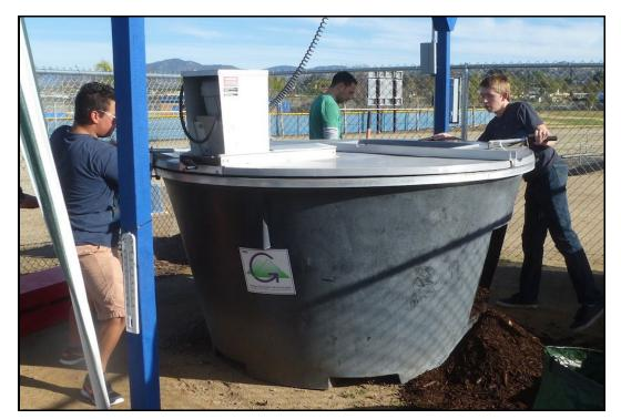
PHOTOGRAPH 8 In-vessel Composting – Earth Tub
