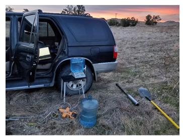
The infiltration tests were conducted in a 3 inch diameter test hole, at depths of 2 to 3 feet deep. The approximate locations of the infiltration test holes are indicated on the attached Infiltration Location Map, Plate 1. Infiltration test holes were located by property boundary measurement on the site plan and/or by using geographic features. The test holes were filled with water and allowed to stand for an extended period of time.
