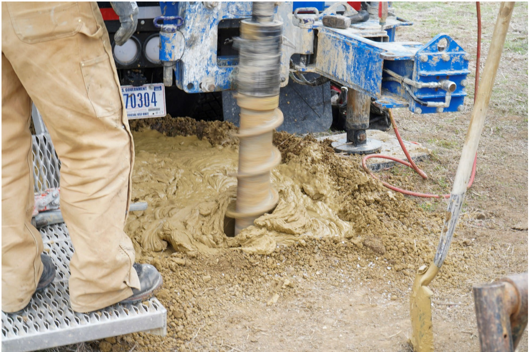
Photo 4 – Representative photo of rotary auger boring.
