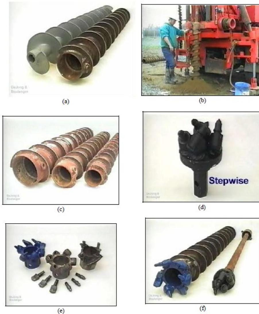
**Figure 1: Hollow Stem Continuous Auger Drilling Systems: (a) Comparison with solid stem auger; (b) Typical drilling configuration; (c) Sizes of hollow stem auger flights; (d) Stepwise center bit; (e) Outer bits; (f) outer and inner assembly. (After FHWA, 2002)**
