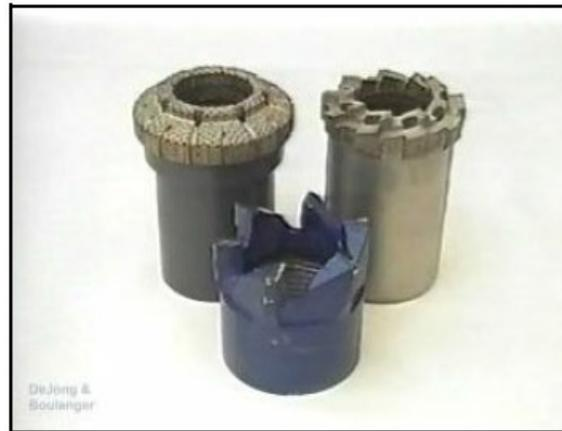
Figure 4: Coring Bits. From left to right: Diamond, Carbide, & Sawtooth. (After FHWA, 2002)
