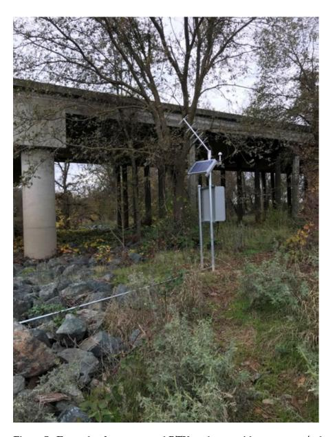
Figure 7. Example of a constructed RTU enclosure with an antenna/solar panel mast.
